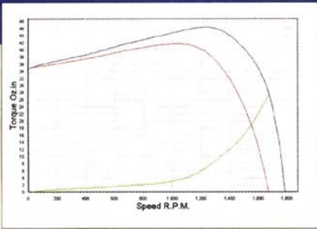
Figure 1. Load Extraction: The load's torque-speed curve (in green) is the difference between the motor's torque-speed curve (in blue) and the motor + load torque speed curve (in red).
